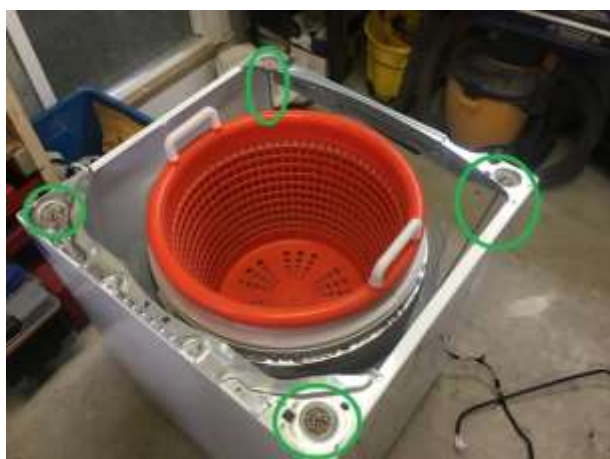
Figure 4 - Support de la cuve
